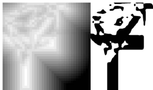
Figure 19: A randomly generated SDF (left) and its rasterization (right) which maximized the predicted score for \boxed{F} (1.893 out of a nominal 1.0) while scoring all other letters low. Parts are recognizable as an \boxed{F} , but other parts are fully bonkers. This is actually one of the least weird ones.
