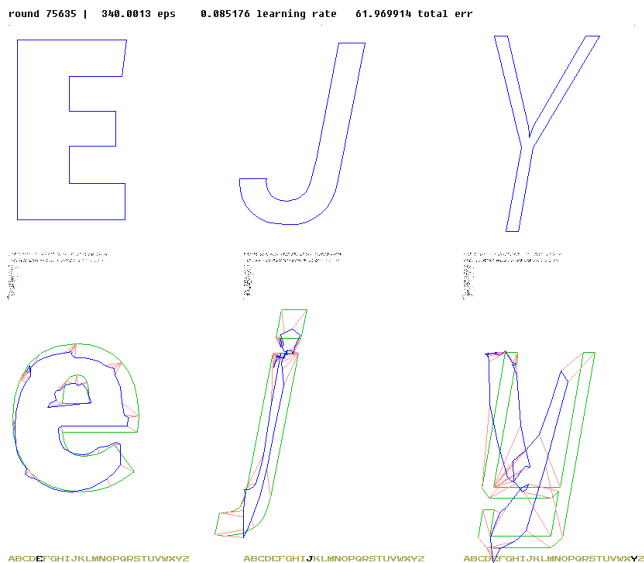
Figure 8: Screenshot (somewhat compacted) of training from near the final round of the vector model’s training, illustrating the permissive loss function that finds the best alignment. At the bottom are the predicted lowercase shapes (blue), also shown with their expected shape (green). We require each point to be mapped (red) to a point from the expected contour in a monotonic order (but several can be mapped to the same one), so that we can attribute error to each point.
